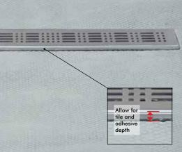
The grate needs to be flush with the tiled surface (tile + adhesive). Raise the whole drainage channel using the 2mm and 4mm self-adhesive spacers.
