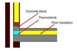
Waterproofing: Although when sealed together Thermoblock creates a permanent waterproof barrier, Thermoblock is not classified as a DPM. A separate Damp Proof Membrane should therefore be included in the detail. The DPM can be fixed directly above or below the Thermoblock but because Thermoblock is waterproof, typically it is fixed above the Thermoblock layer.
