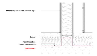
Variations to the above examples can be used – masonry or timber frame wall Insulation can be above or below the slab – in whichever case, Thermoblock is below the level of the screed.
